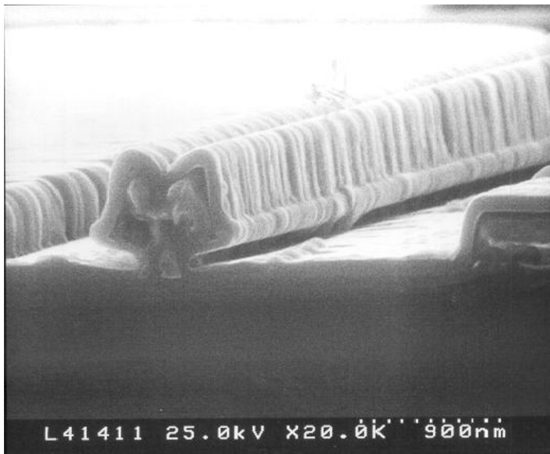
Figure 3-6 The SEM image of the T-shaped gate.
