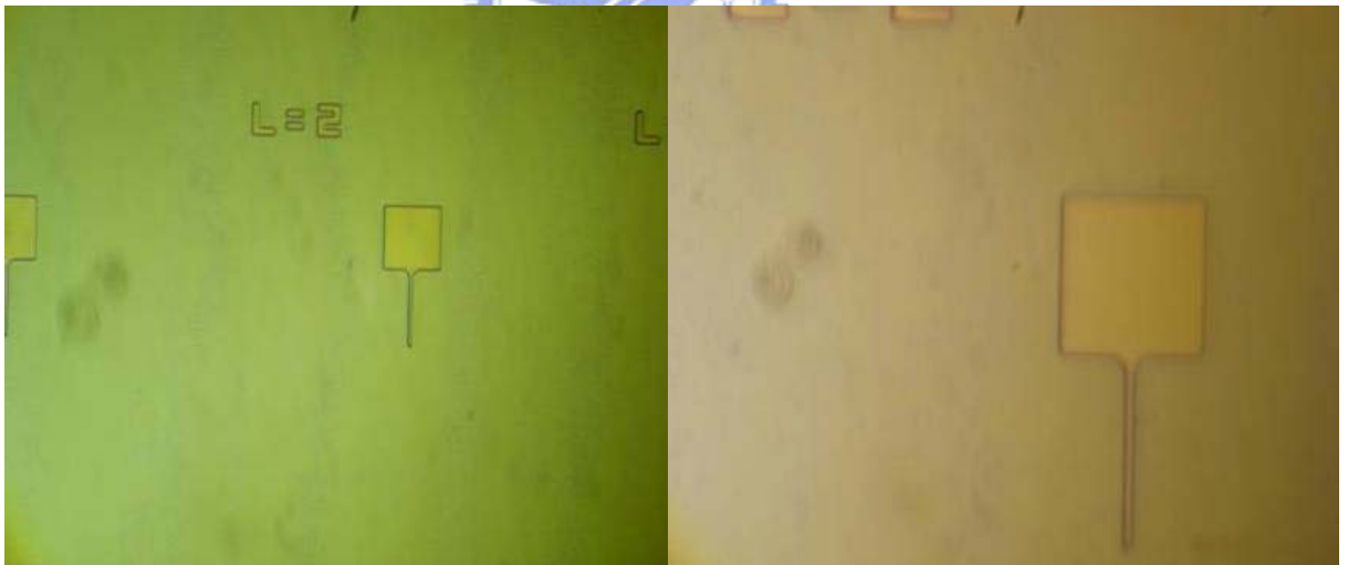
Fig. 4-5 OM images of self-aligned implantation devices after lithography. The channel length was 2\mu\text{m} .
