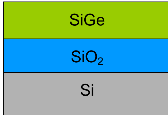
Fig. 2-1. Cross sectional view of SiGe-based P-MOSFET after mask #1.
