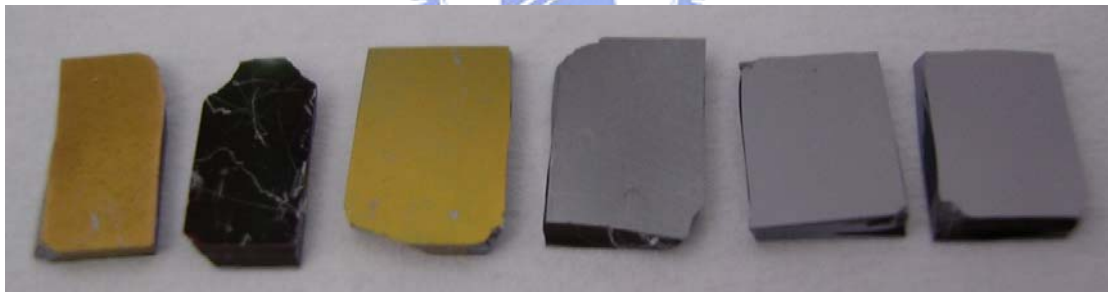
Fig. 2.4 The close photographs of SiO 2 /Si wafer fragments of different level assembly process. (right 1) blank SiO 2 /Si wafer fragment. (right 2) Au NPs on SiO 2 /Si wafer fragment. (right 3) CdSe NPs + Au NPs on SiO 2 /Si wafer fragment. (right 4) Au NPs + CdSe NPs + Au NPs on SiO 2 /Si wafer fragment. (right 5) CdSe NPs + Au NPs + CdSe NPs + Au NPs on SiO 2 /Si wafer fragment. (right 6) Au NPs + CdSe NPs + Au NPs + CdSe NPs + Au NPs on SiO 2 /Si wafer fragment [14].
