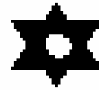
Figure 4-2 Two-pass algorithm in 2D. The binary input image is shown as the right star image. The first pass accumulates the distance value from top-left to bottom-right, while the second pass accumulates the distance value from bottom-right to top-left.
