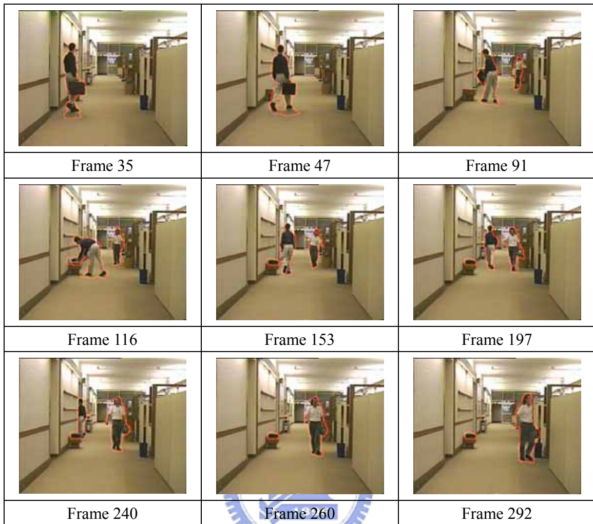
Figure 3-11 Apply the “active contours without edges” model to the hall sequences. Frame 1 is taken as the background. Multiple objects are successfully identified based on the level set approach.
