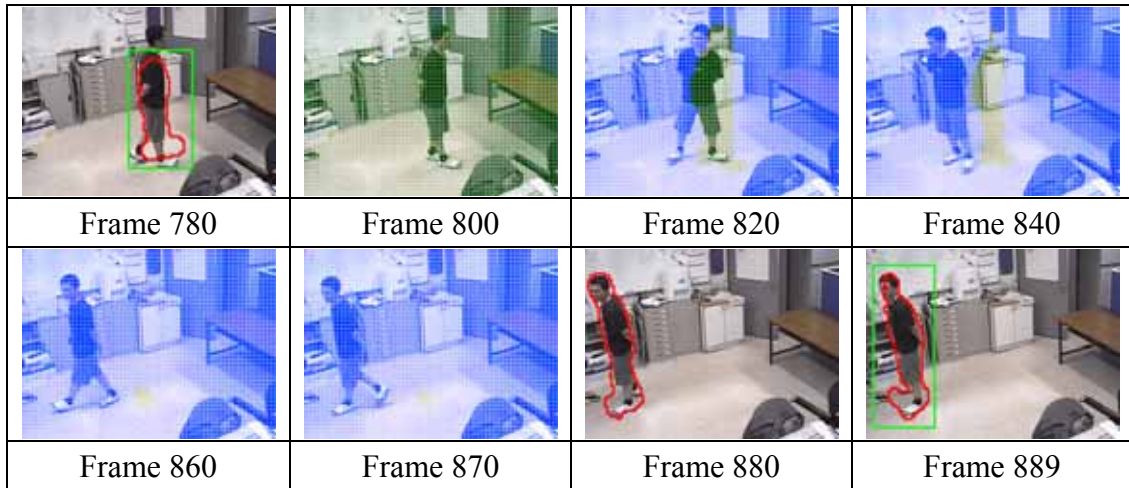
Figure 4-17 The simulation result of Figure 4-16. The images with green grid and blue mask are in the background modeling status. When the background is modeled in all blocks, a background subtraction result is obtained. The frames with a green rectangle represent the tracking results.
