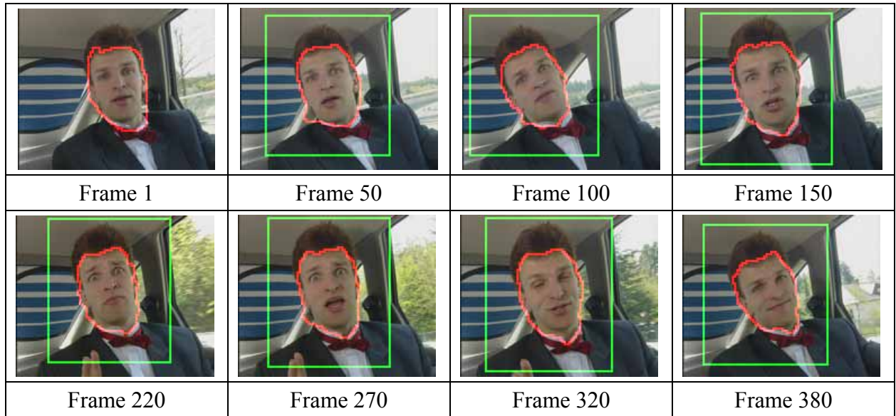
Figure 3-16 The car-phone test sequences. The face region is defined in the first frame. The level surface is only updated inside the green rectangle. The face is successfully tracked even though the scene changes outside the car.
