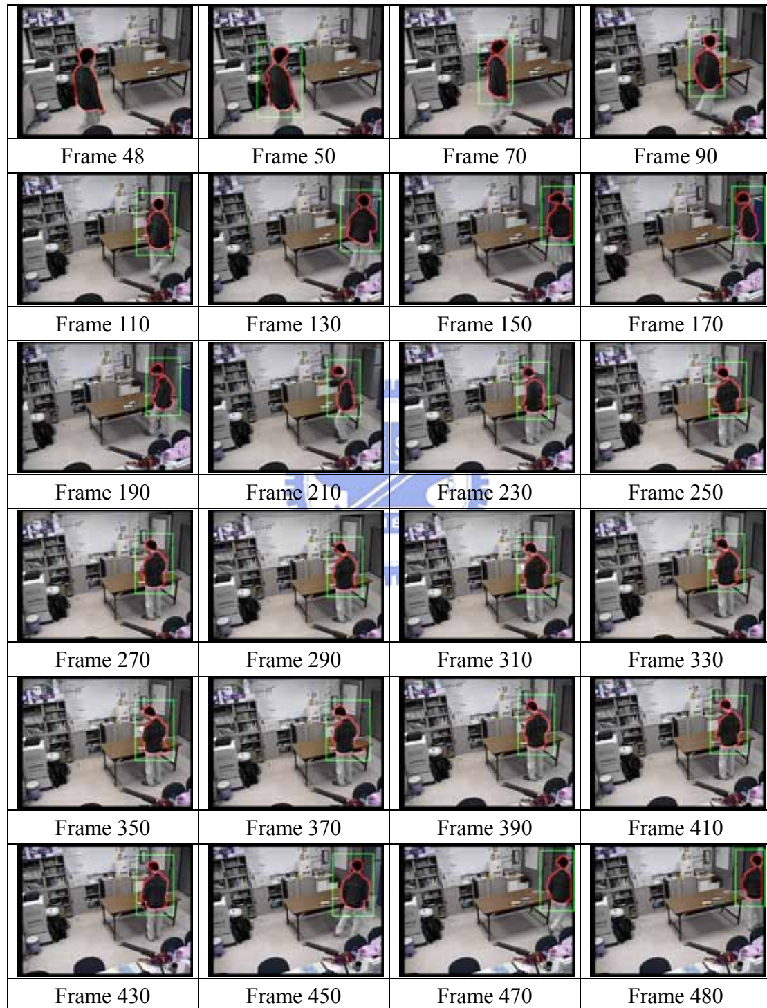
Figure 3-28 The experimental result of real sequences acquired in the laboratory. The contour of the person is preset in the first frame.
