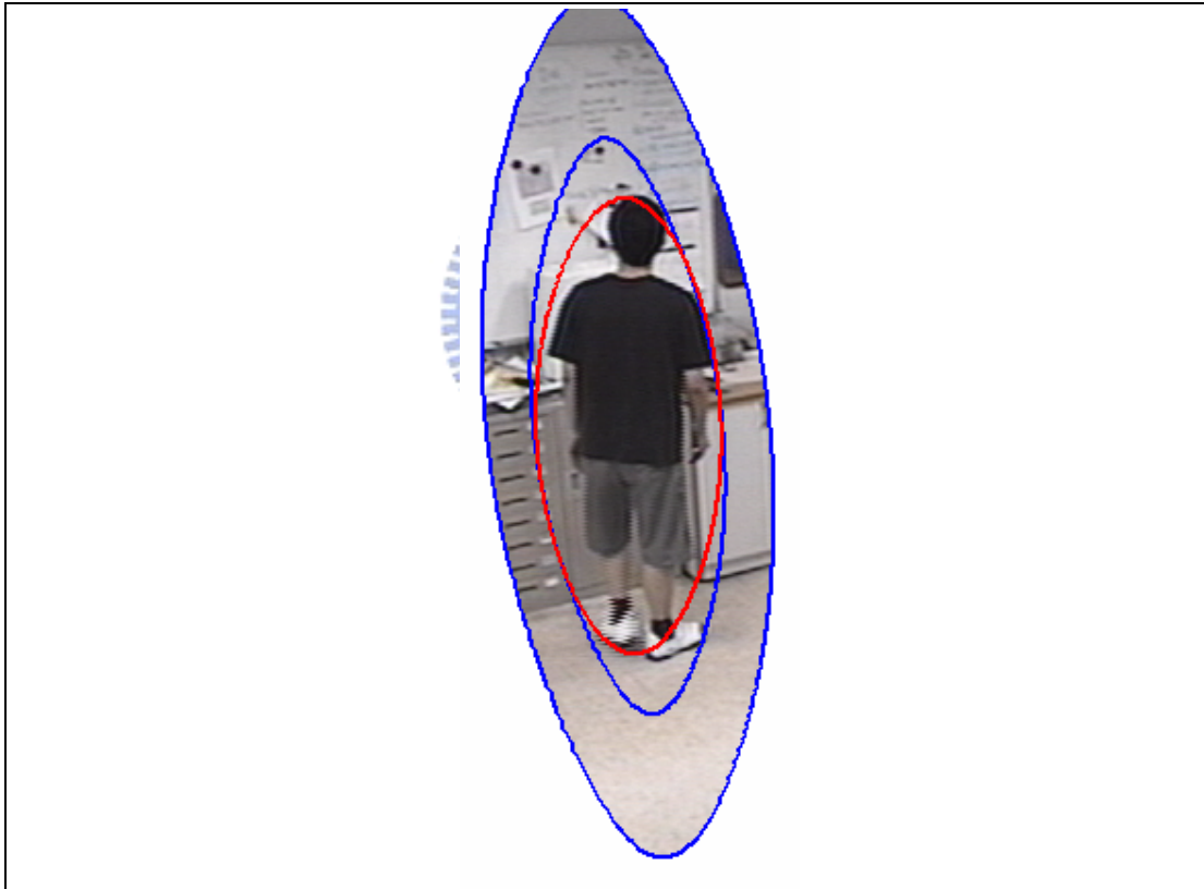
Figure 3.15 Result of size and orientation updating. The blue ellipses represent the 2-sigma contour and the 3-sigma contour with respect to the original covariance matrix. The red ellipse represents the 2-sigma contour with respect to the modified covariance matrix.
