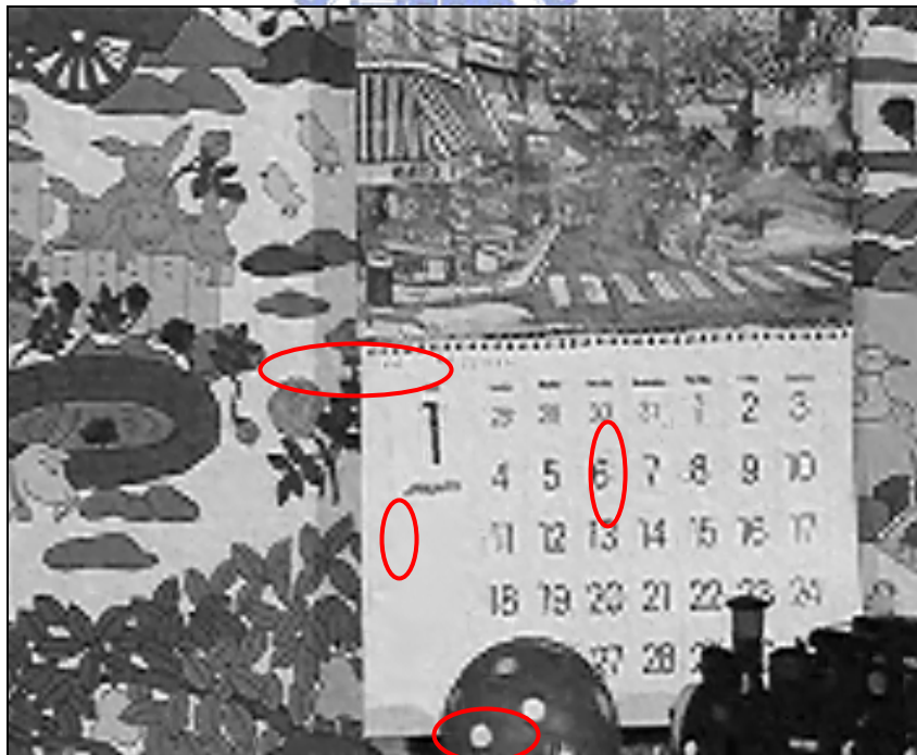
Fig 3.14 Pepper and salt noise in the reconstructed image of the Mobile sequence
