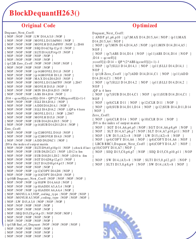
Figure 5.8: Original and optimized assembly code of IQ.
