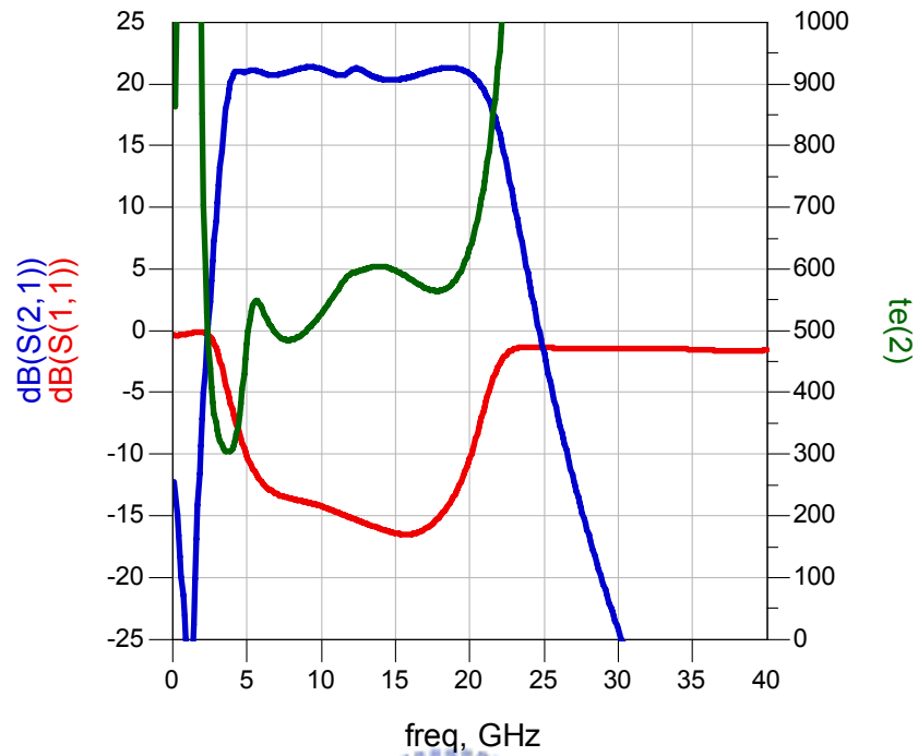
Fig. 3.6 The simulated S-parameters of wide-band low noise amplifier
