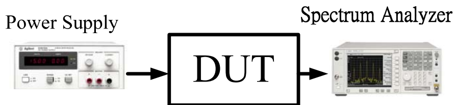
Figure 5.5 Testing setup for the voltage-controlled oscillator.
