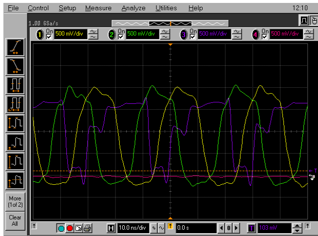
Figure 5.26 Reference frequency later 22ns than divider output frequency
