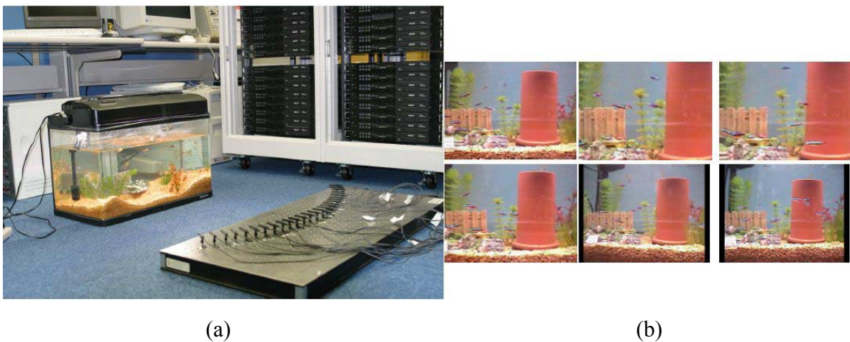
Figure 6.1: (a) Capturing and processing parts of FTV system. (b) Free viewpoint images generated in real time.
