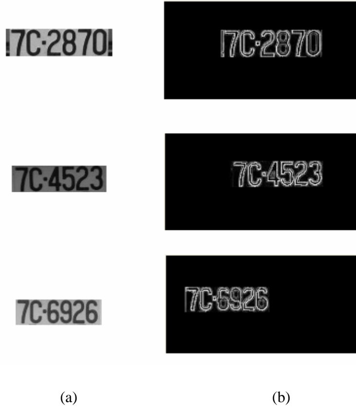
Fig 3.1 (a) the original license plate, and (b) the result of the character edge detection.
