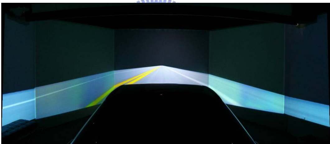
Figure 3-1: The simulated high way scene. The visual information is reduced to minimum to avoid unnecessary stimuli.
