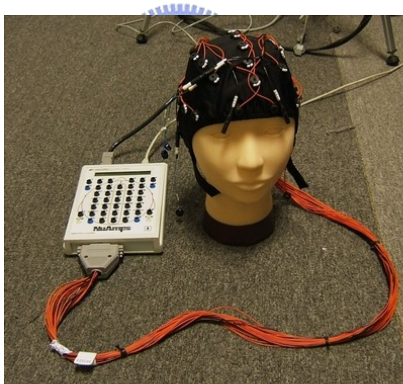
Figure 2-10: The NuAmps EEG Amplifier and the Electrode Cap
