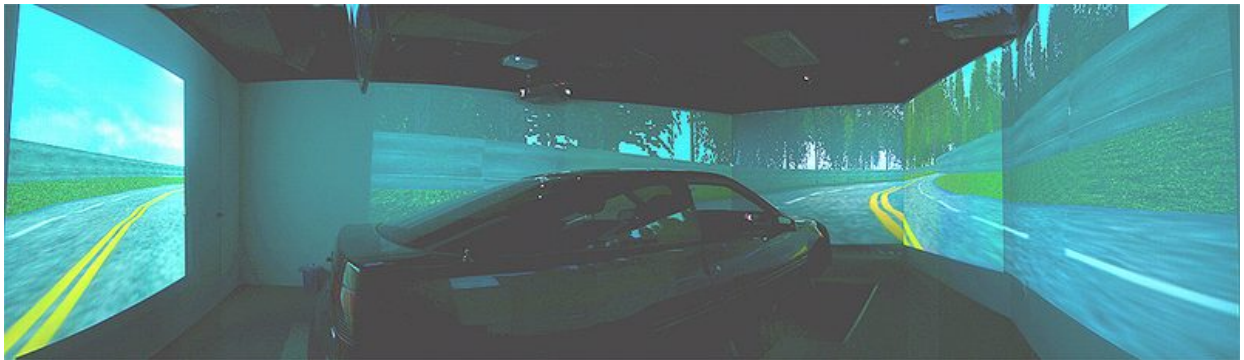
Figure 2-4: The overview of surrounded VR scene. The VR-based four-lane highway scenes are projected into surround screen with seven projectors.
