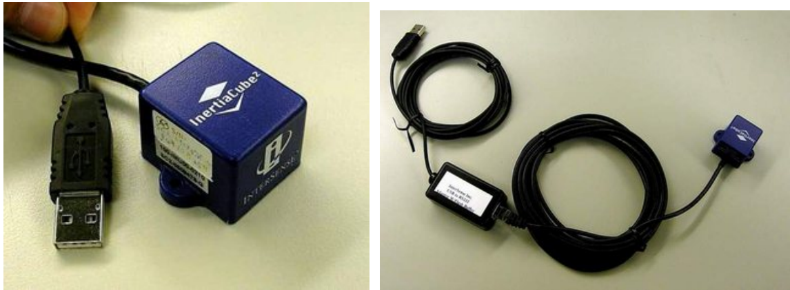
Figure 2-7: The accelerometer or platform motion tracking, Inertia Sensing, InertiaCube 300
