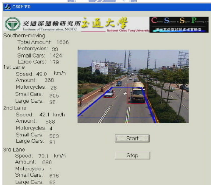
Fig. 5-8 Results of vehicle detection and traffic parameter calculation in the urban.
