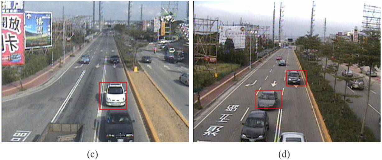
Fig. 5-11 Stopped vehicles are detected and split by the proposed methods of queue detection and resolution.
