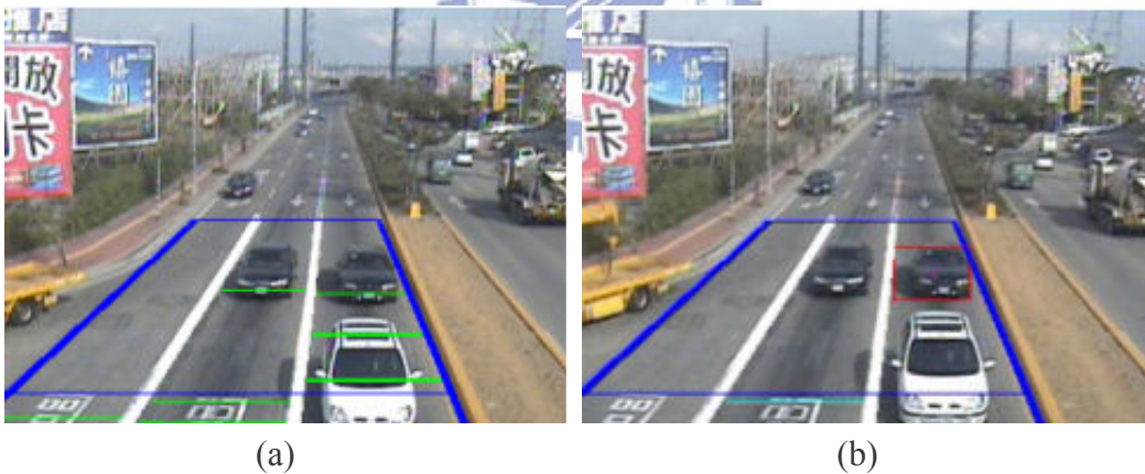
Fig. 4-14 The fake green split line located on a vehicle sunroof in (a) is removed in (b).
