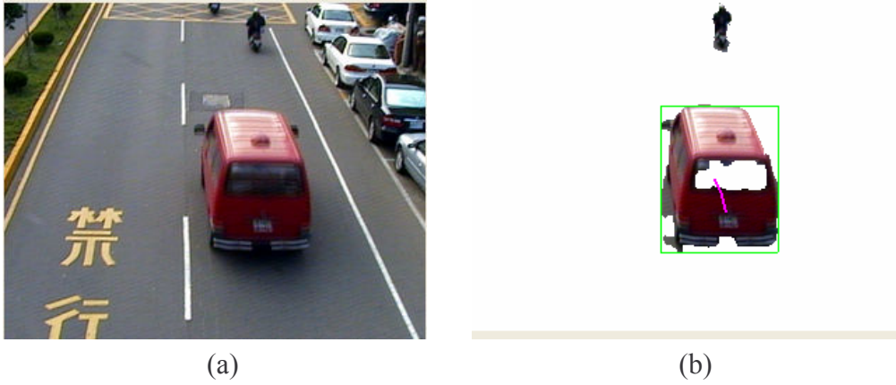
Fig. 3-6(a) The original image (b) The moving object image that middle part of moving object is eliminated.
