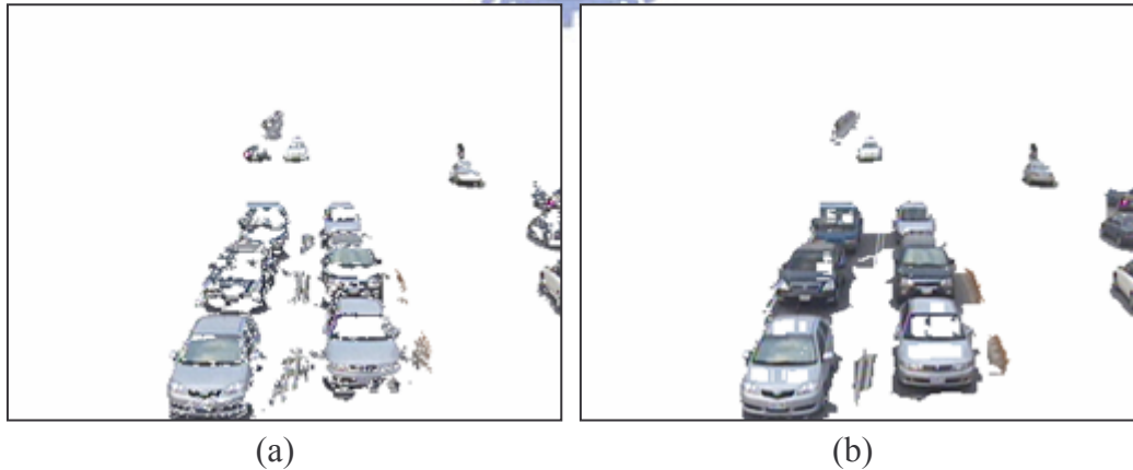
Fig. 3-12(a)The detected vehicles are fragmented with inexact shadow judgment. (b)The detected vehicles are with some shadows which are not eliminated clearly.
