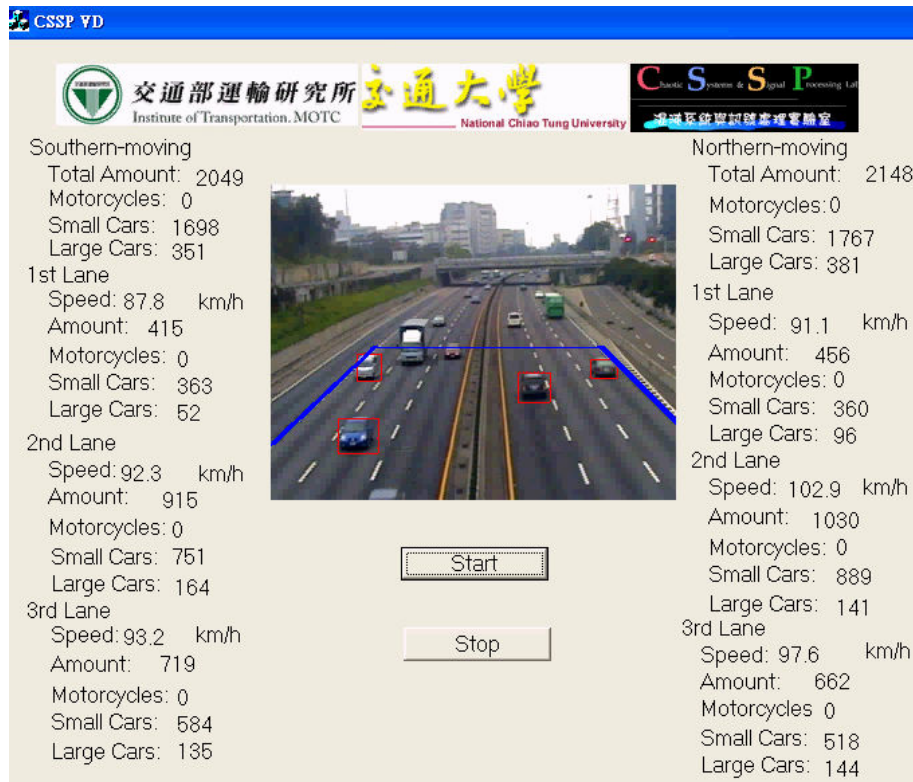
Fig. 5-7 Results of vehicle detection and traffic parameter calculation in the expressway.
