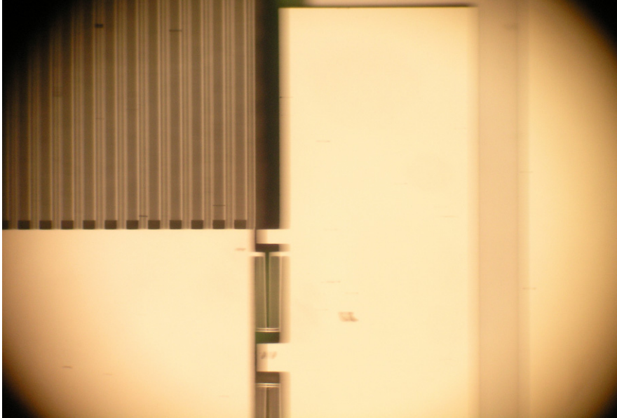
Figure 4.7 Device resonance at 156 Hz with maximum displacement
