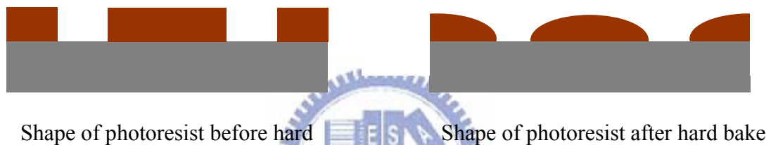
Figure 3-6: The shapes of PR before and after hard bake
