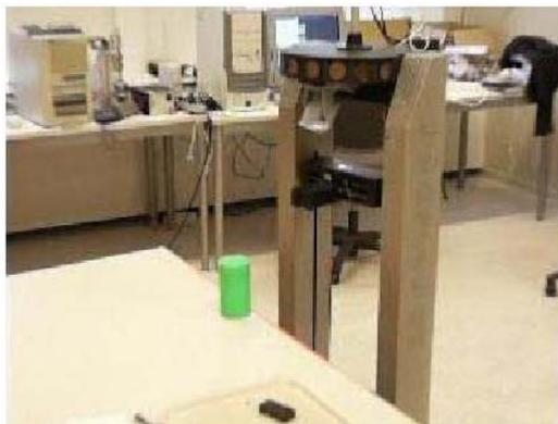
圖 1.2 Pan-tilt camera and 1-DOF robot arm [2]
