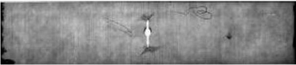
Fig. 10 X-ray examination of [90_2/\pm 45_2/0_2]_S laminate at 95% of failure load
