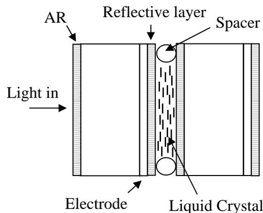
Fig. 3.2 Liquid-crystal Fabry-Perot étalon filter [55]. AR: anti-reflection coating
