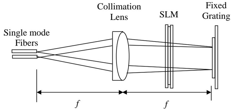
Fig. 3.4 The tunable wavelength filter by combining a SLM and a fixed grating [59]. SLM: spatial light modular;  $f$ : focal length
