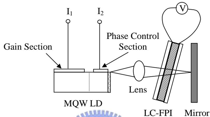
Fig. 3.3 ECDL uses a LC-FPI and a MQW laser diode [57]. MQW: multi-quantum-well; LD: laser diode
