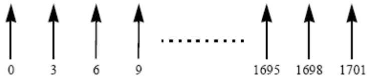
Figure 2.8: Example of DL preamble for segment 1
