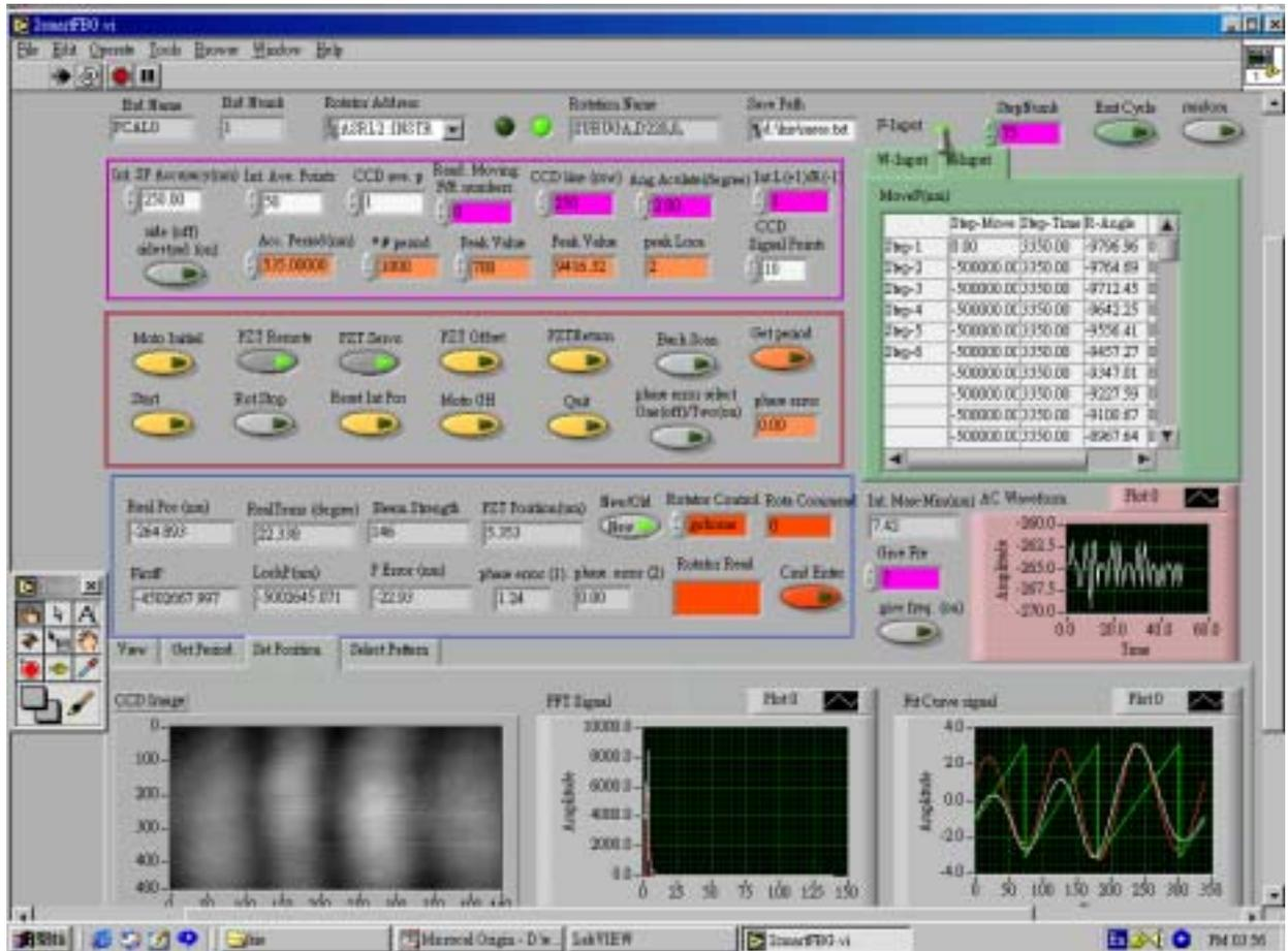
Fig. 4.31 The Labview program of side-diffraction monitoring method for fabricating long FBG.
