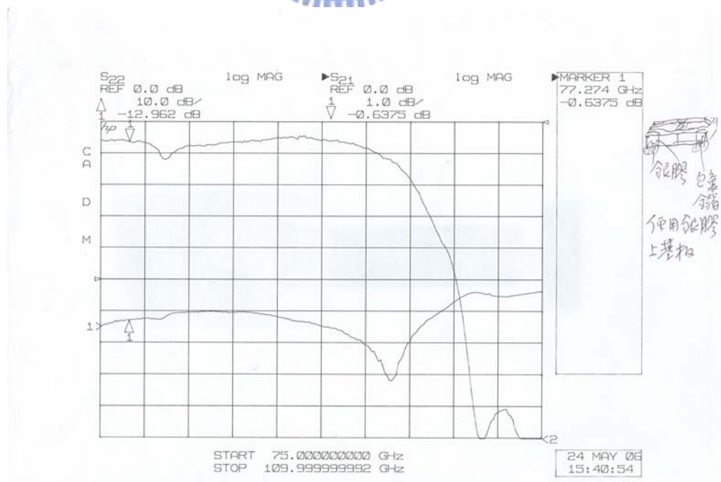
圖 2-23 77GHz cpw-mstrip transition test (back-to-back)
