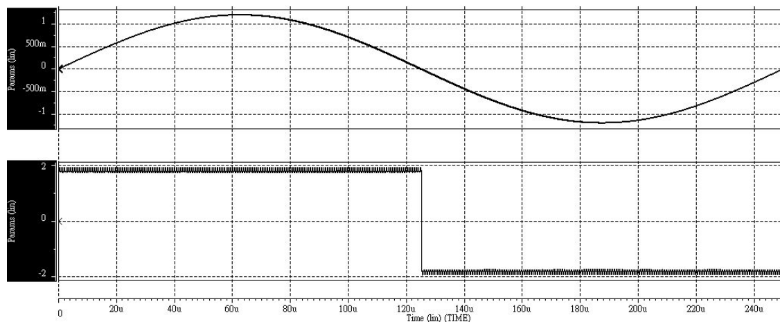
Figure 4.11 Simulation result of comparator
