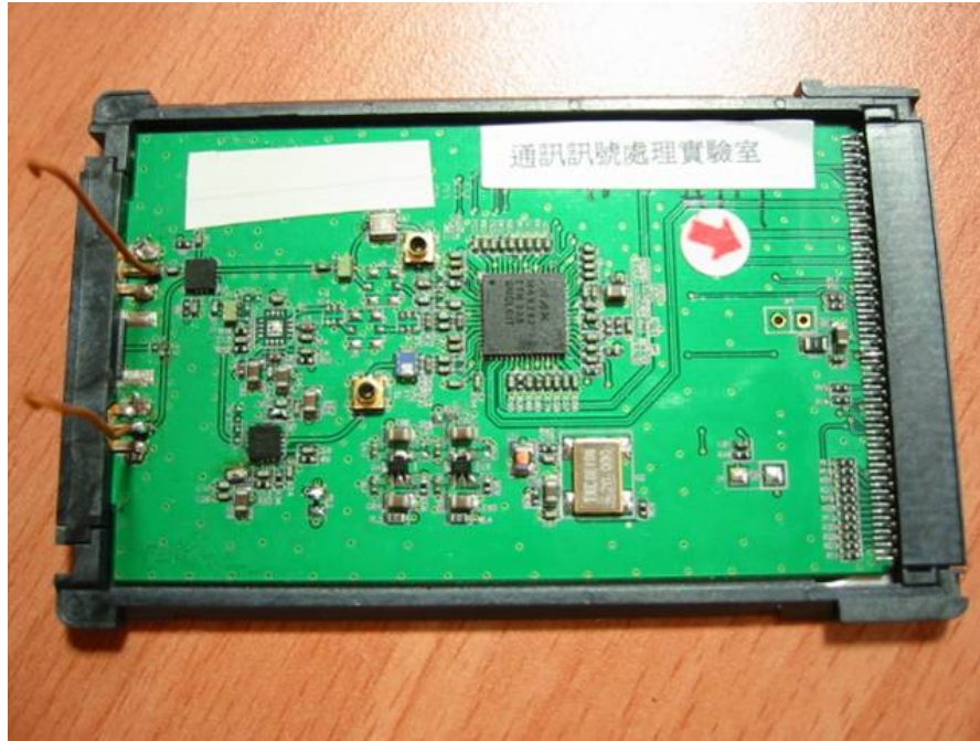
Figure 3.13: RF module on self-designed platform
