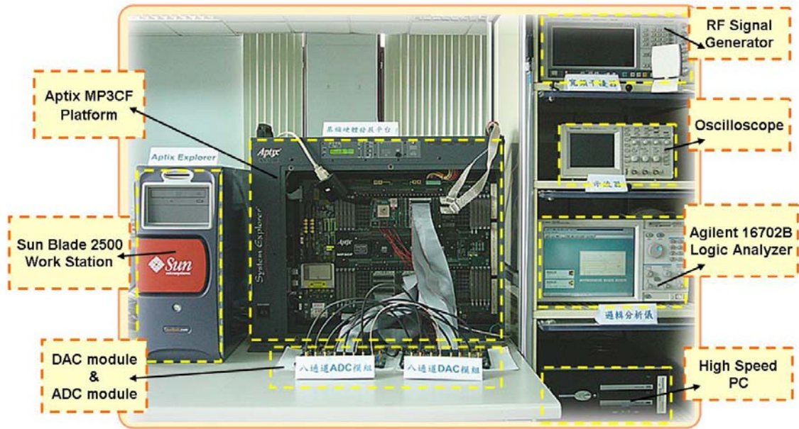
Figure 3.1: Development environment of fast prototyping system
