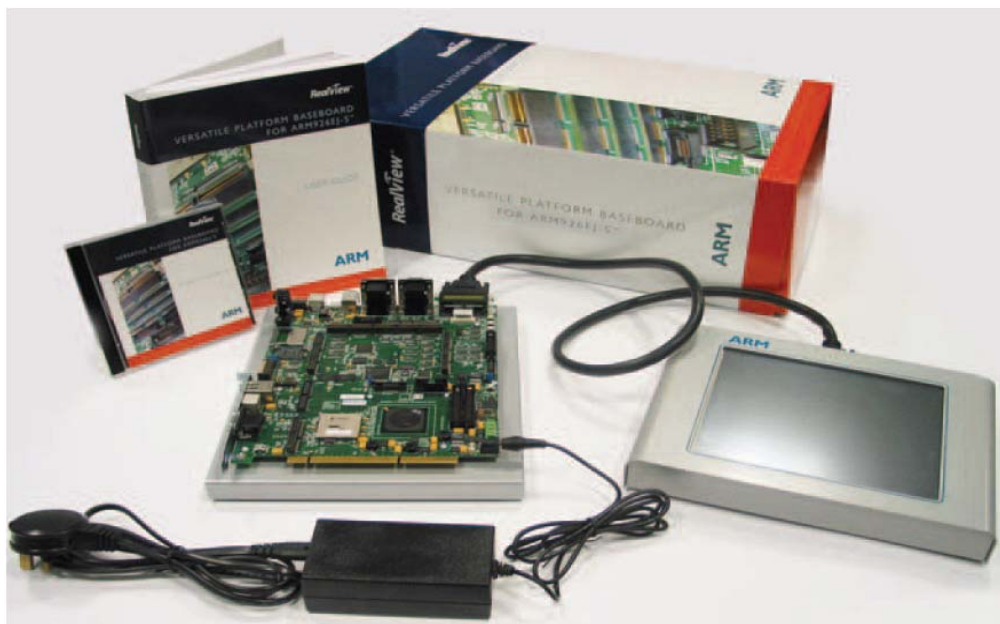
Figure 2.4.1: Versatile Platform Baseboard for ARM926EJ-S
