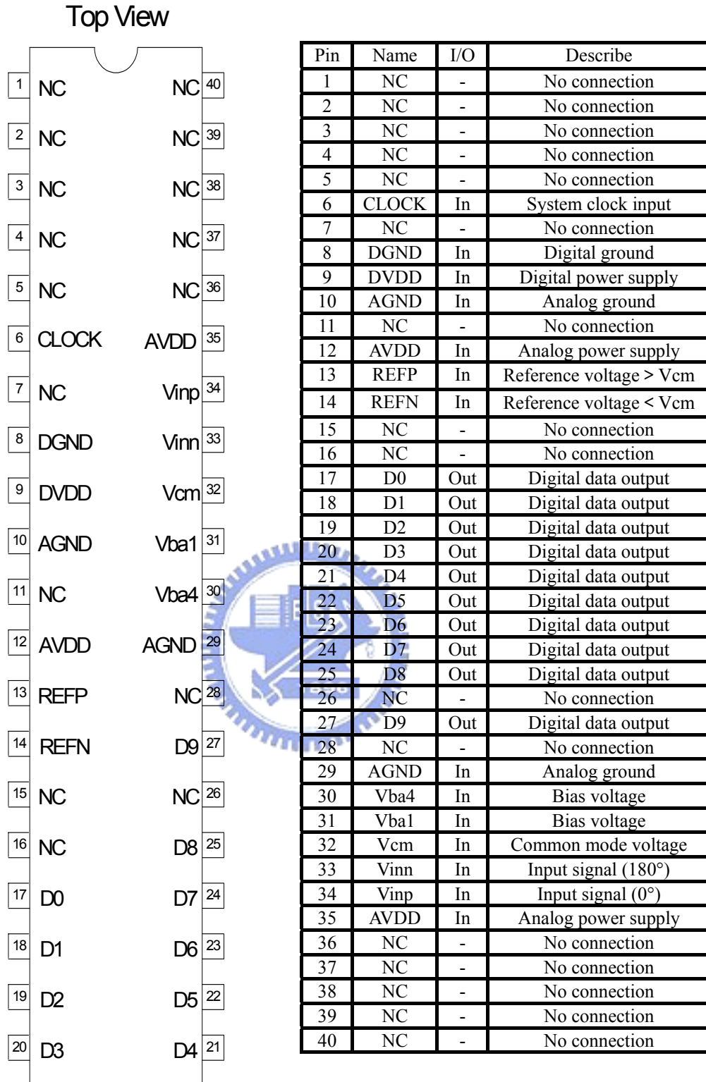
Figure 5.11 (a) Pin configuration diagram and (b) Pin assignment
