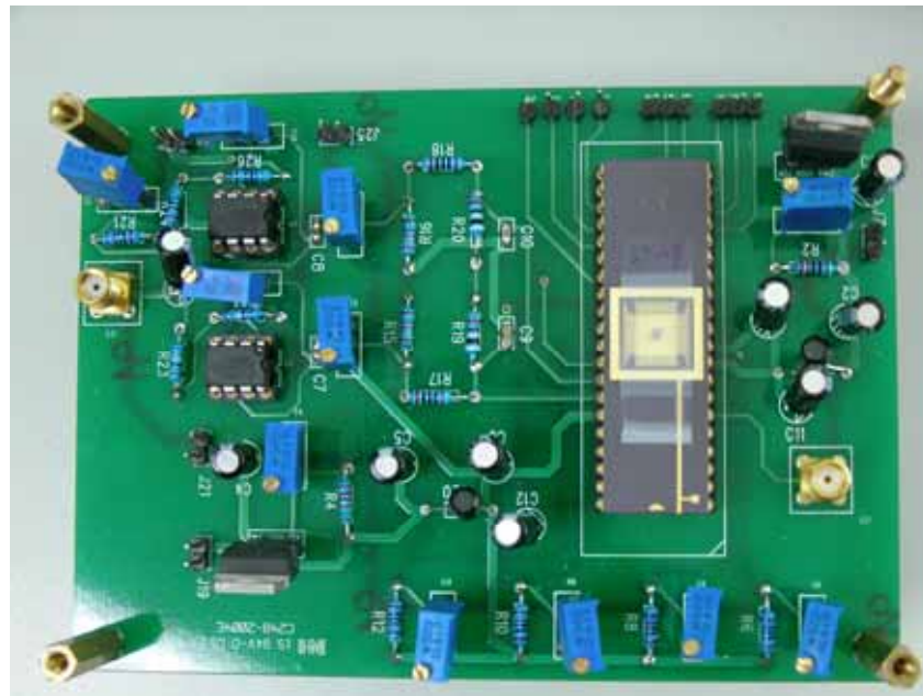
Figure 5.2 The photograph of the experimental pipelined ADC DUT board
