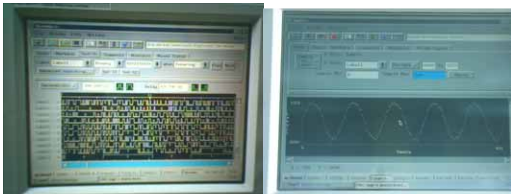
Figure 5.13 Measured results for 150 Msample/s conversion rate (a)Output bit streams (b) Plot chart
