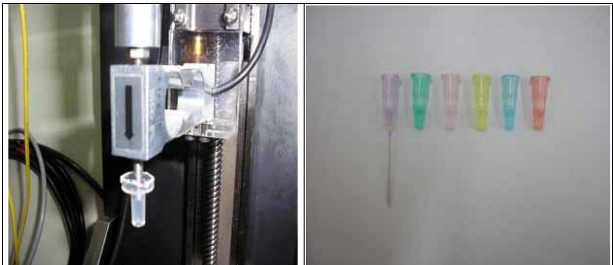
Figure 24 Needles fixture
