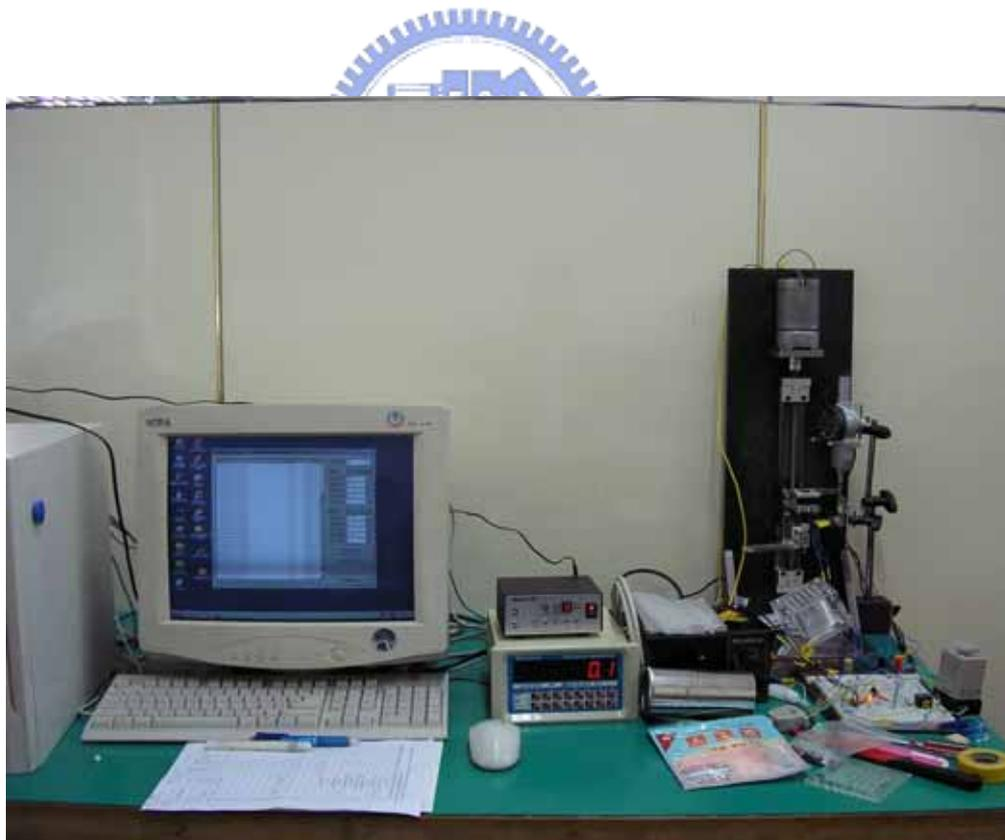
Figure 20 Set up of insertion force measure equipment
