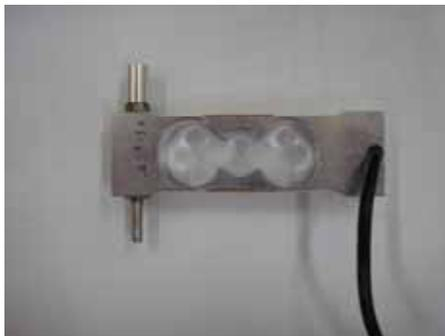
Figure 21 Load cell
