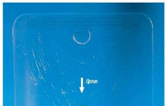
Jetting on a flat transparent part
