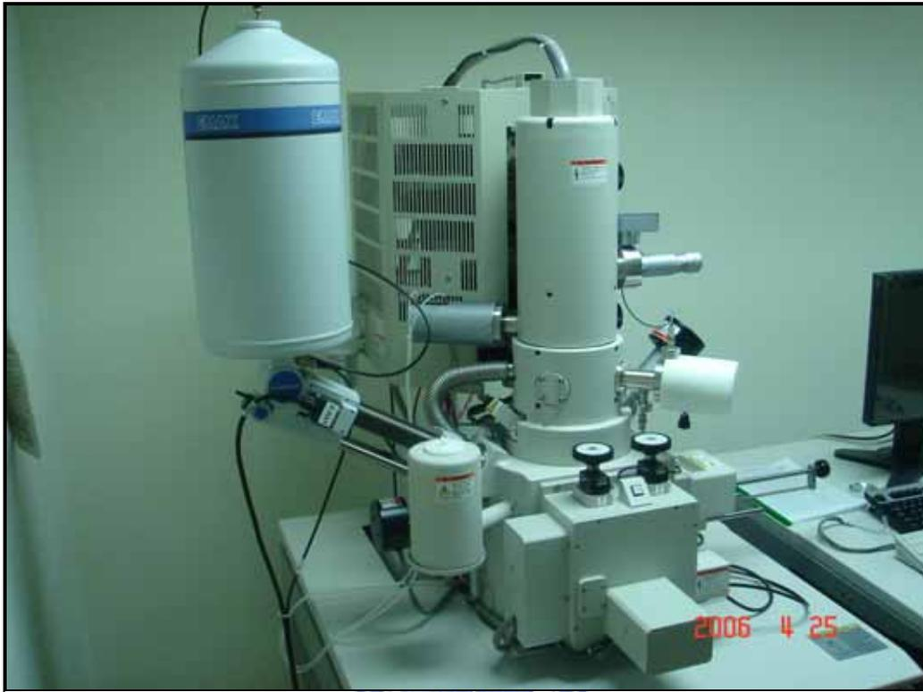
▲圖 3-9 Hitachi S-4800 Scanning Electron Microscope
