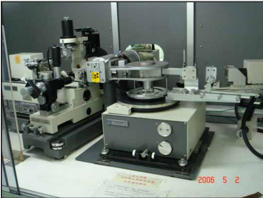
▲圖 3-10 Siemens D-5000 X-ray Diffractometer
