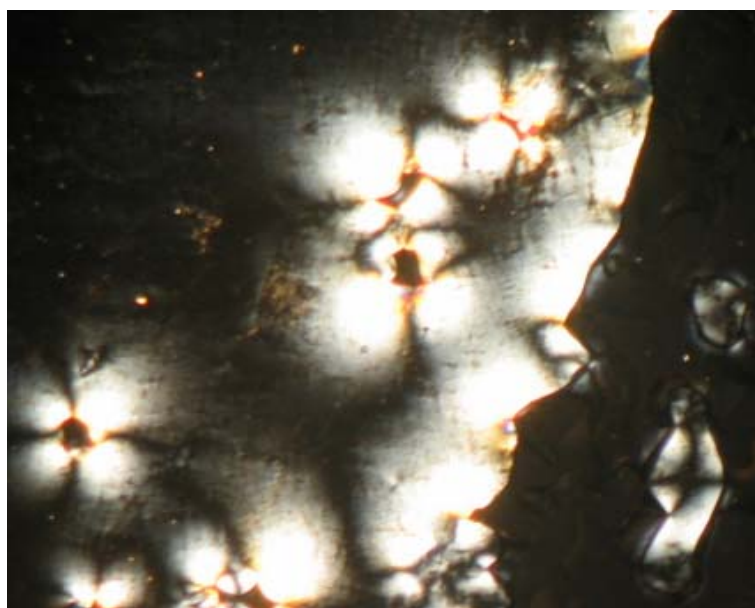
Fig. 3-15 Polarizing optical micrograph of polymer PF1 at 175 °C
