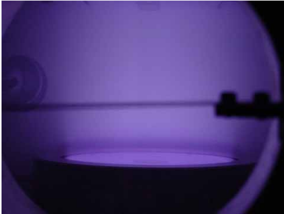
Figure 4.19. The discharge was operated without the magnetron assembly in the pressure 90 mtorr
