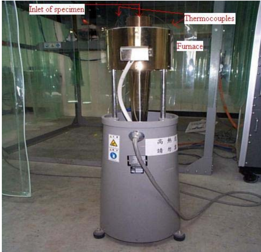
Figure 2.13: An elementary material test apparatus
