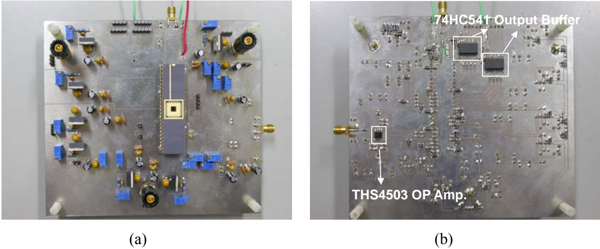
Figure 2. 17 (a) Top view of the testing board (b) bottom view of the testing board.
