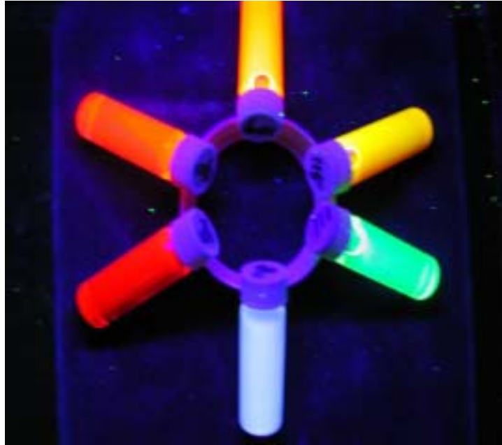
Figure 1.2 Size-dependence of the PL color for colloidal solutions of CdSe QDs passivated with a ZnS shell. The smallest ( \sim 1.7 nm) CdSe QDs emit blue, the largest ( \sim 6 nm) QDs is red emission.
