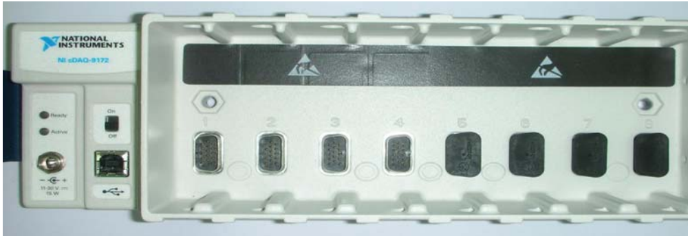
(a) Picture of the CompactDAQ Chassis.
