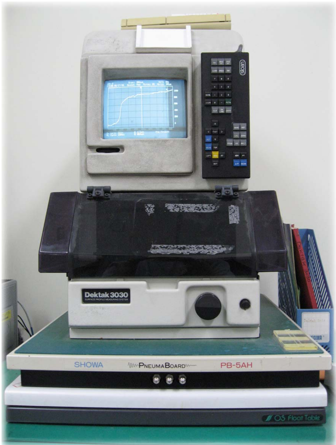
Figure 3.18. The configuration of surface profilometer (Sloan Dektak 3030 profilometer).
