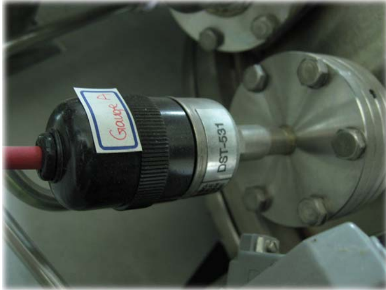
Figure 3.11. The configuration of thermocouple gauge.
