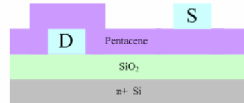
Fig. 3.8 Different bias in TBC structures (a) TBC bot-source and (b) TBC top-source
