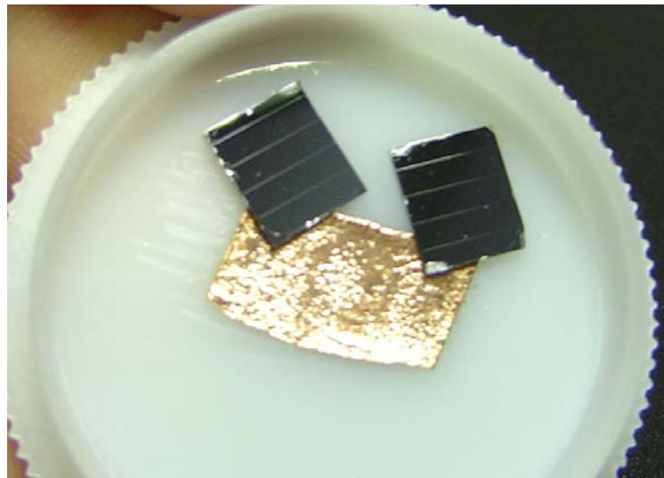
Figure 4.2 A top view of two bonding structure samples after channel patterns defined.
