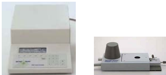
Fig. 3.3 Instrument photos of center controller (left one) and hot stage (right one)
