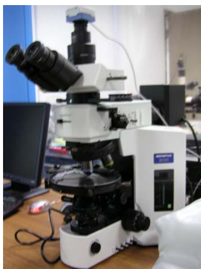
Fig. 3.2 Instrument photo of POM, OLYMPUS BX51.
