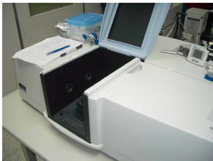
Fig. 3.4 Instrument photo of UV-VIS Spectroscopy, LAMBDA 650 PerKin Elmer.
