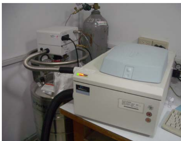
Fig. 3.1 Photo of PerkinElmer diamond DSC and its liquid nitrogen cooling system.
