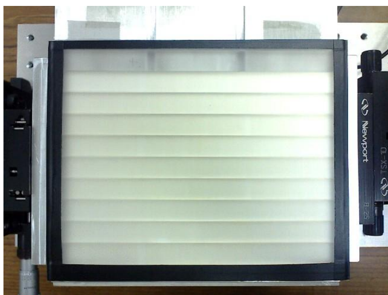
[Fig. 4.1] FSC LCD backlight system
