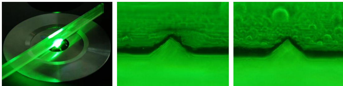
[Fig. 4.3] The micro-groove profiles measured under the optical microscope
