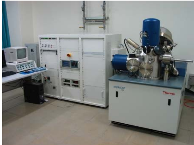
Fig. 4.2 X-ray Photoelectron Spectroscopy (XPS), VG Scientific, Microlab 350
