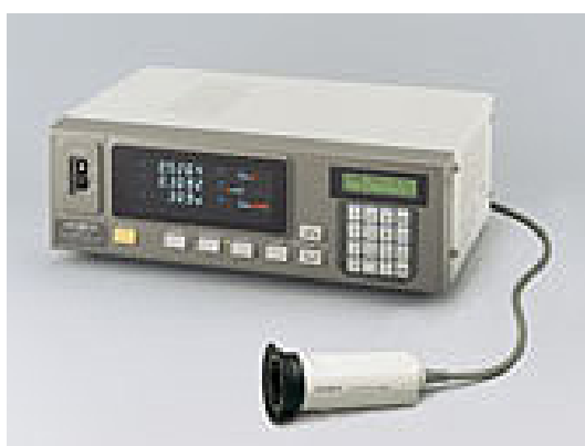
Fig. 3.13 Color analyzer CA-100 used in this work. Panel performance such as luminance, color temperature, color coordinate can be measured by this apparatus.
