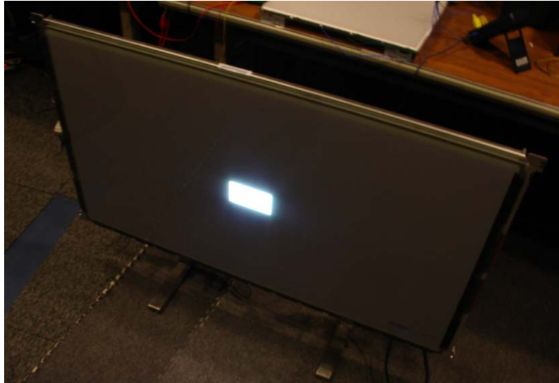
Fig. 4.6(a) The optical measurement system using for the image sticking observation. CA-100 is used to record luminance, color coordinates, and color temperature of the selected pattern.
