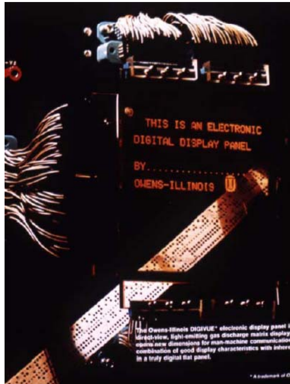
Fig. 2.8 Open-cell structure was used in this 128 by 128 pixel plasma display developed by Owens Illinois in 1968 which measured 4-in by 4-in. It consisted of a robust 6-mm-thick glass substrate, thick film gold electrodes, and a screen printed solder glass dielectric layer [14].
