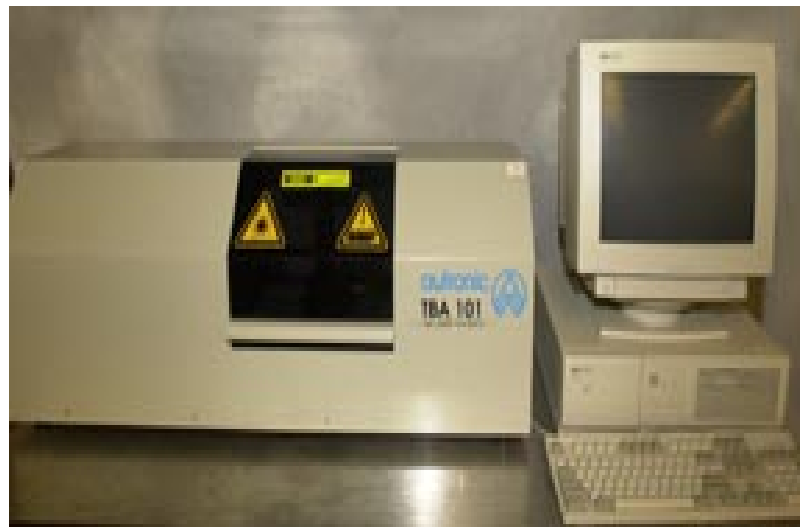
Fig. 3-5 Pretilt angle measurement system (Autronic DMS 101 TBA)
