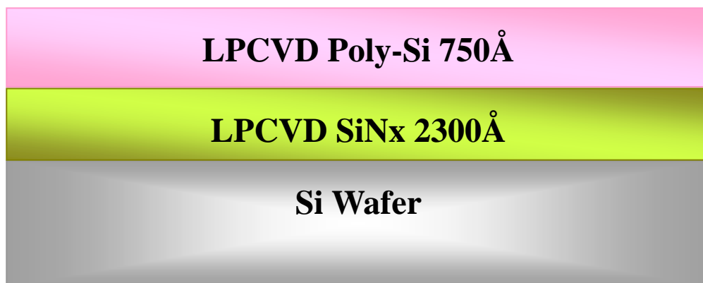
Fig. 2-2 Cross-sectional view of polycrystalline silicon thin film
