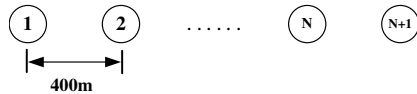
Figure 5.1: The network topology used to evaluate the performances of UDP/TCP multihop connections
