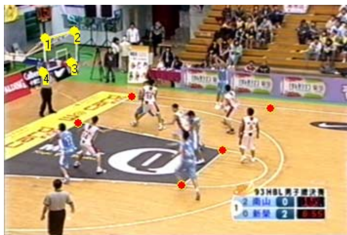
Fig. 4-3 The 2D location of the points for camera calibration and the backboard position.
