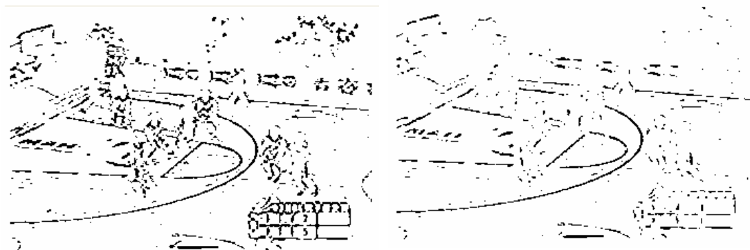
(c) Extracted white line pixels without line-structure constraint. (d) Extracted white line pixels with line-structure constraint.
