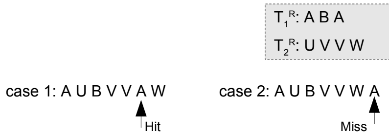
Figure 2.3 Illustration of how interleaving accesses from another task determines whether the access will be a cache hit or cache miss, assuming a 4-way full associative cache.
