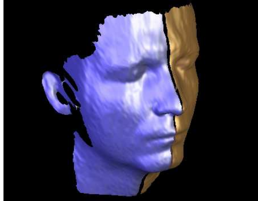
Figure 1.2: 3D Laser Scanning Result of A Human Face. "A reconstruction result of human face using 3D laser scanner." source: ( http://www.muellerr.ch/engineering/laserscanner/default.htm )
