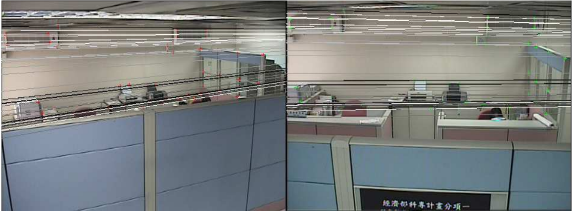
Figure 6.7: Scene 1 - Epipolar Lines Calculated With The Fundamental Matrix.
