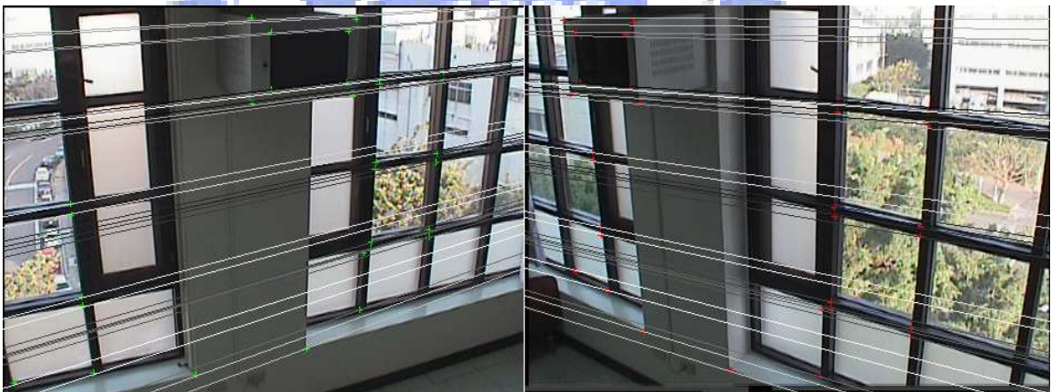
Figure 6.8: Scene 2 - Epipolar Lines Calculated With The Fundamental Matrix.
