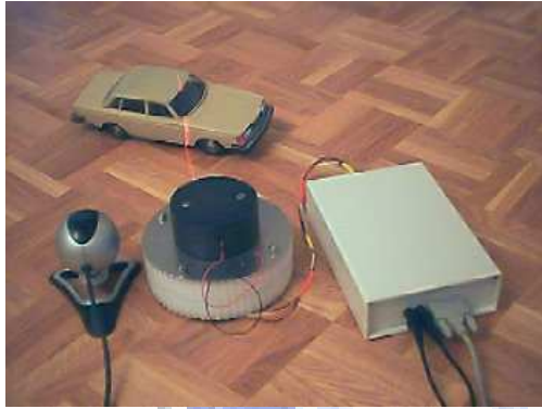
Figure 1.1: A 3D Laser Scanner. "A 3D laser scanner which scans in the depth data in order to rebuild virtual objects of real ones." source: ( http://www.muellerr.ch/engineering/laserscanner/default.htm )
