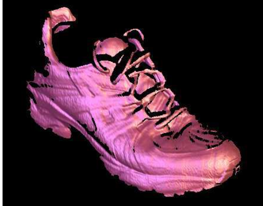
Figure 1.3: 3D Laser Scanning Result of A Shoe. "A 3D rebuilding result of a shoe using 3D laser scanning data." source: ( http://www.muellerr.ch/engineering/laserscanner/default.htm )
