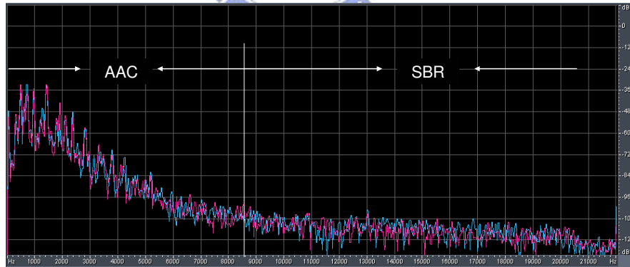
Figure 28: The envelope comparison between high bands and low bands. The envelope of high bands is flat, and the envelope of low bands is sharp.
