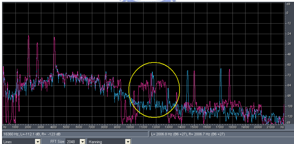
Figure 31: Noise floor overflows due interpolation mode. The target circle indicates the noise floor overflow is from the averaged energy with tone component.
