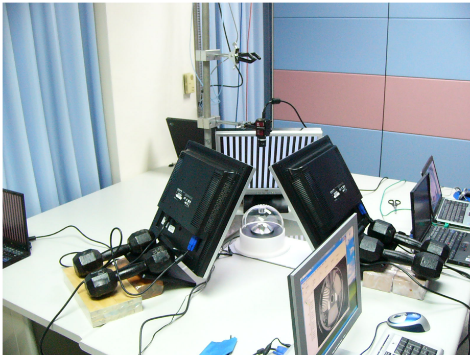
Figure 4.9: Setup of the LCD for non-central catadioptric camera calibration.
